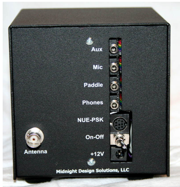
Figure 2: The rear of the SDR Cube contains the usual complement of I/O connectors, including a specialized one for optimized use of the NUE-PSK modem for digital modem support.
