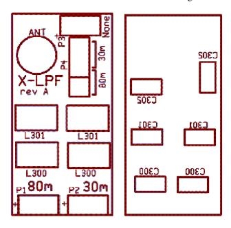
**NOTE:** Yes, we know the bottom side text designators (above-right) are reversed. Unavoidable. The board silkscreen is correct, of course. Please just follow the silkscreen labels on the board if you have trouble reading **sdrawkcab**.
